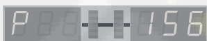
Shaft is positioned at any other position. This value can lie between 0 and 255 and changes with the rotation of the shaft.
