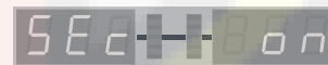
The balance run can be started only when the wheel guard is closed.
