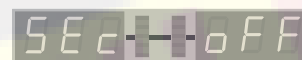
The balance run can be started only when the wheel guard is closed. If the hood is opened during the measuring run the motor is switched off and the wheel runs free. This function is useful to view the run out of the wheel. As soon as the hood is closed again the measurement run will start again from the beginning.
