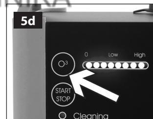
If the LED light is in 'High' position and the  $O_3$  button is pushed, it moves to 0 position.
