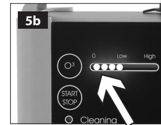
LED lighted on 'Low' position. Ozone treatment 15 min. Immediately after this ozone treatment, the treatment with the Air Purifier liquid will start. This position is chosen for strong smell problems.
