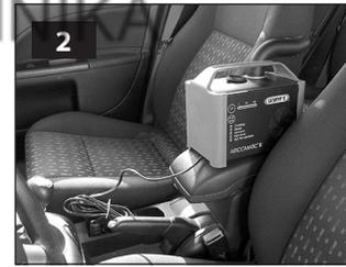
Put the machine horizontally upright on a convenient place in the middle of the car interior.
